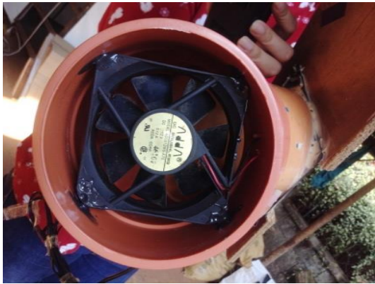
Installation of 12V DC Fan inside the Pipe
