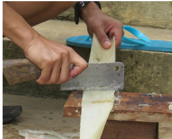
EXTRACTION OF THE BANANA SHEATH
