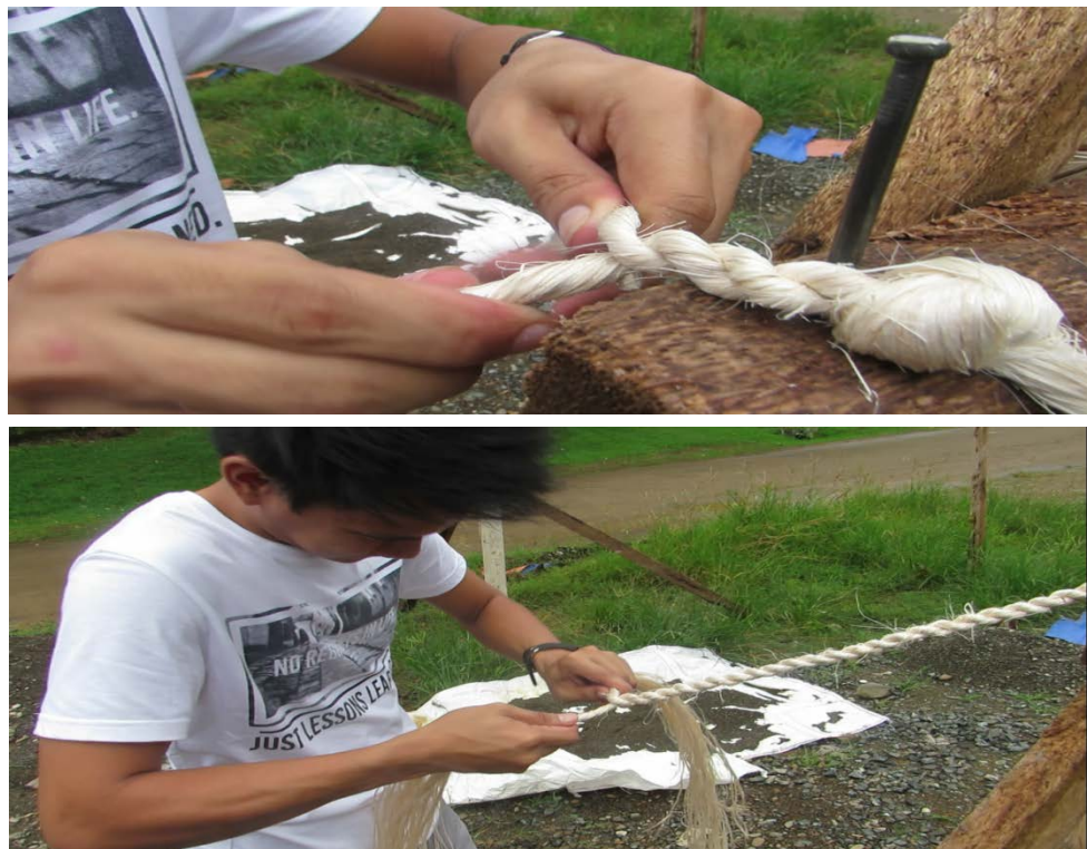
TWISTING THE BANANA FIBER
