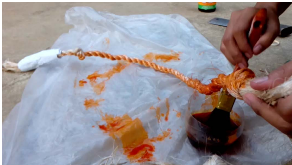
APPLYING THE VARNISH
