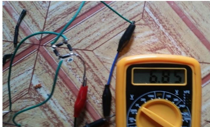
Figure 3.24. Measuring the Rectified Voltage of the Piezoelectric Disc
