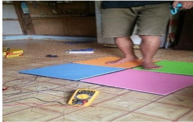
Figure 3.23. Harvesting Human Footstep Energy
