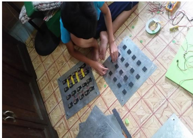
Figure 3.19. Mounting of Rubber Pieces and Piezoelectric Discs
