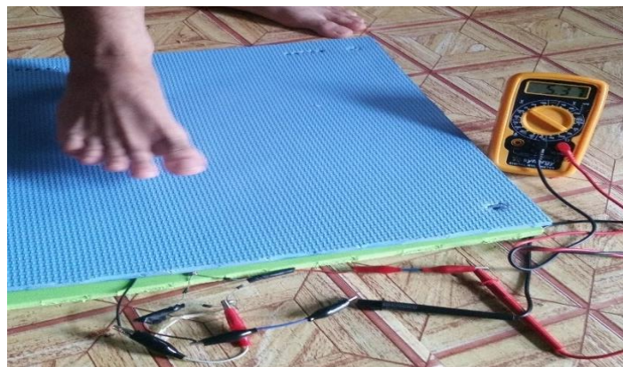
Figure 3.32. Testing and measuring of the output of the first design
