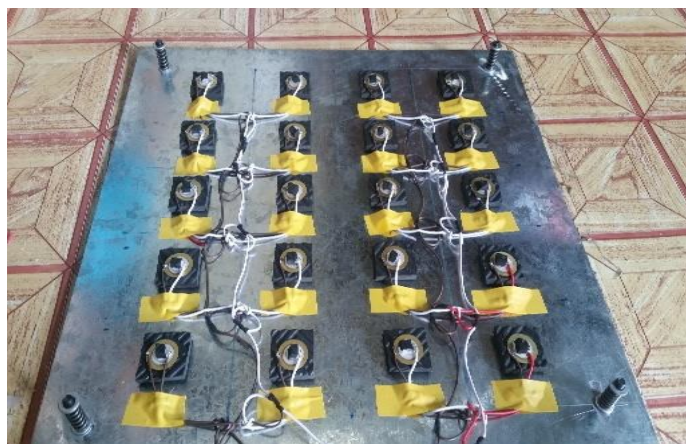
Figure 3.20. Assembled Arrays of Piezoelectric Discs
