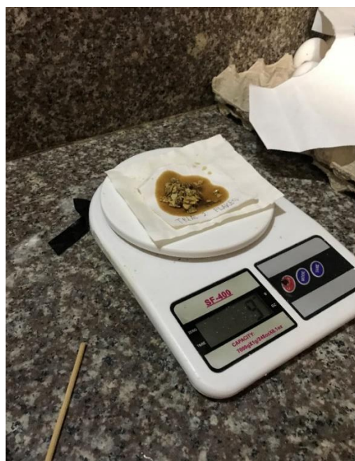
Weighing of sorbent after suspension
