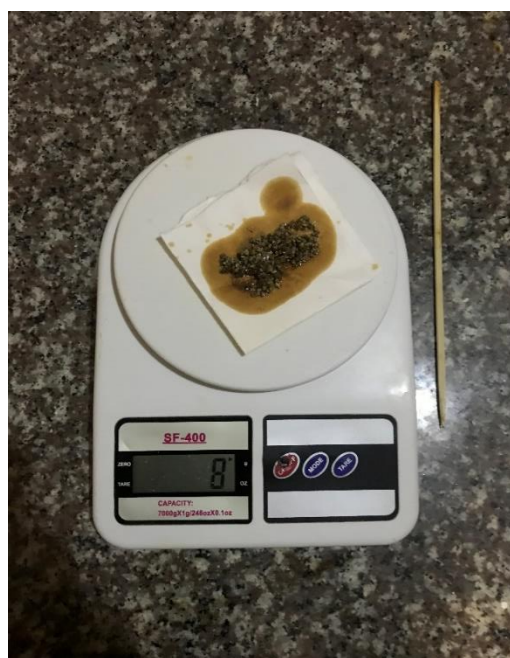
Weighing of sorbent after suspension
