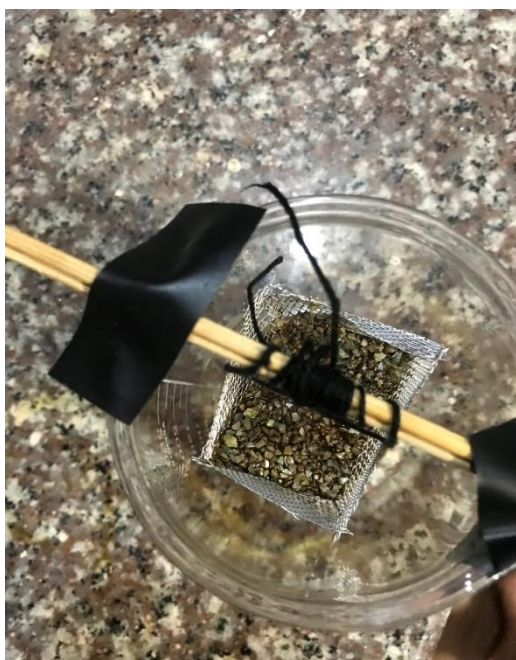
Suspension of Sorbent for 30 minutes
