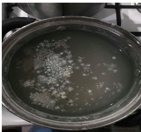
Heating of powdered shells in NaOH solution
