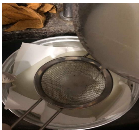
Draining-off the NaOH solution
