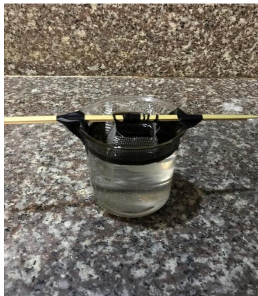
Soaking of sorbent with bunker oil and water for 15 minutes
