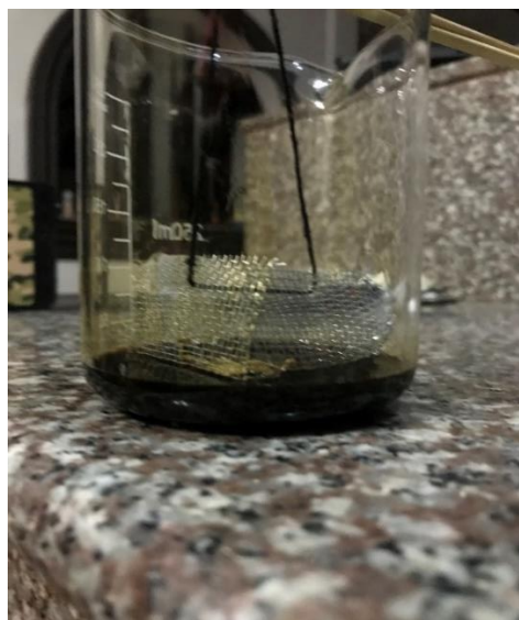
Soaking of sorbent with bunker oil for 15 minutes
