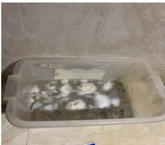
Soaking of shells in HCl solution
